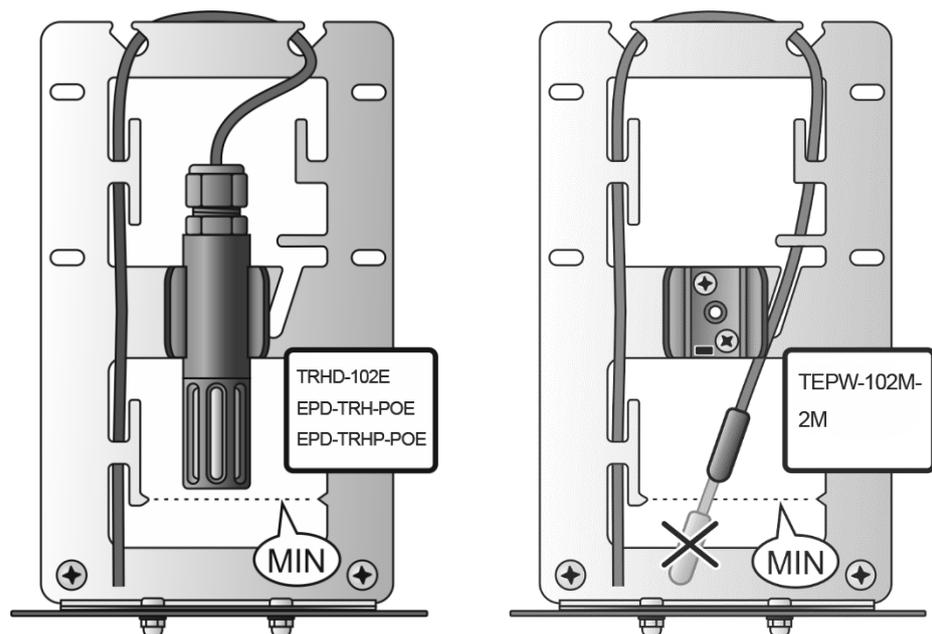
If the probe cable is too thin (approx. 2 to 3 mm, eg for the AT-TG3 probe) and there is a risk of instability of the probe sensor, secure the probe cable by turning the probe holder. See pictures below.
